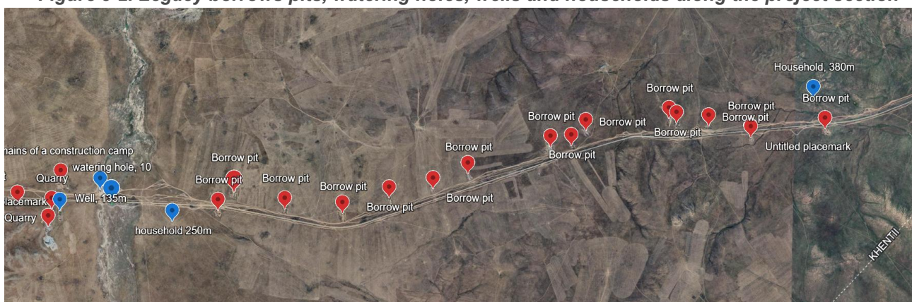
Figure 3-2. Legacy borrows pits, watering holes, wells and households along the project section
